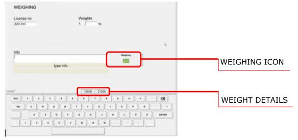
Finally, the driver accepts the weighing by pressing the weighing icon on the touchscreen, whereby the device prints out the ticket.
