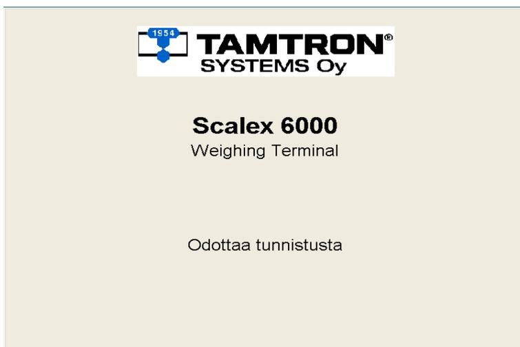
Terminal display when the boom is closed and there is no truck on the weighbridge.
